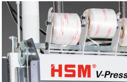
Manual bale strapping with continuous polyester tape
