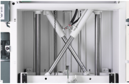
Quick and easy installation due to crossed cylinders
