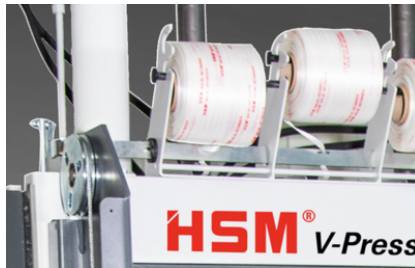
Manual bale strapping with continuous polyester tape
