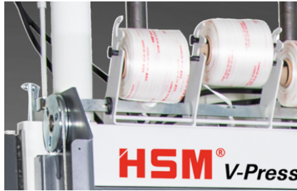
Manual bale strapping with continuous polyester tape
