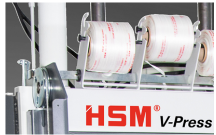
Manual bale strapping with continuous polyester tape
