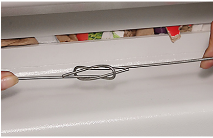
Manual bale strapping with wire
