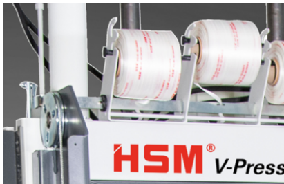
Manual bale strapping with continuous polyester tape
