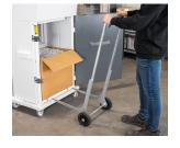
The removal trolley allows for the easy removal and disposal of the compact bales.
