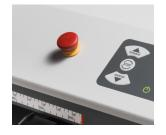
When the emergency stop switch is actuated, the device stops immediately.
