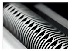
Specially hardened solid steel cutting rollers
