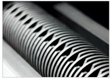
Specially hardened solid steel cutting rollers
