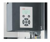
Convenient membrane keypad with text display, which shows the current status of the machine
