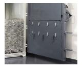
Special retaining claws optimize the compression of the pressing material.
