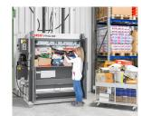
To fill the press, the upper half of the doors is pushed down and automatically opens after the compression process
