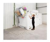
Convenient filling via hydraulic lifting/tilting device
