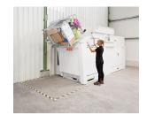
Convenient filling via hydraulic lifting/tilting device
