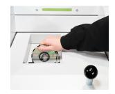
Thin optical, magnetic and electronic data media can be shredded comfortably and quickly using the input slot.
